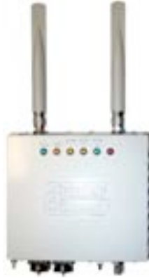
3e-525C-2 Wireless Mesh Access Point / Bridge Node
